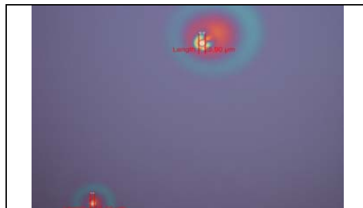
Figure 8. Structures on a ON209 wafer subjected to BHF dip prior to spinning.
