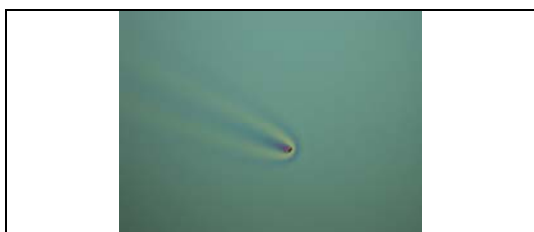
Figure 9. Structure on a pre-treated wafer, spin-coated By Microresist. Defects at the edge of sample.
