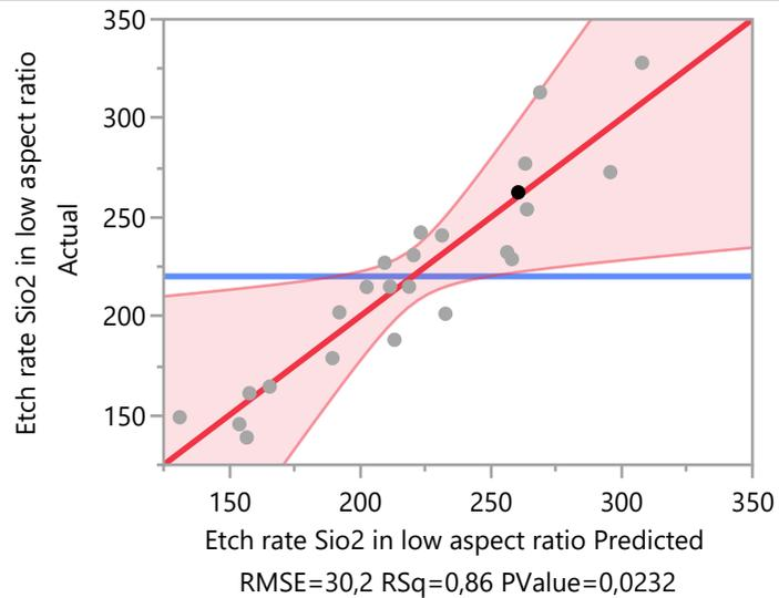
**Least Squares Fit****Response Etch rate Sio2 in low aspect ratio****Residual by Predicted Plot**
