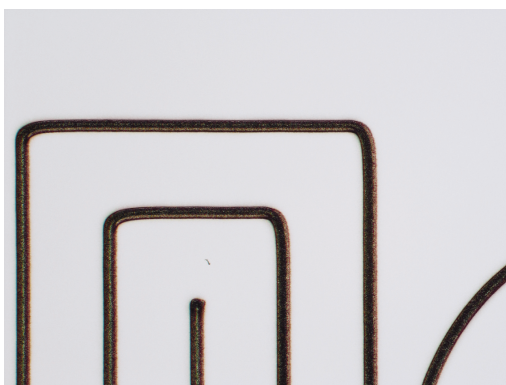
Figure 47: Polygon delay too short, resulting in rounded corners.
