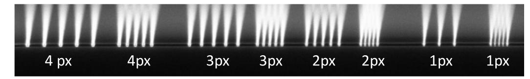
We test high resolution patterning by writing single and multipixel lines in approximately 50 nm thick resist. We do this to detect process inconsistencies. Under normal conditions we consistently pattern 12 nm lines.
