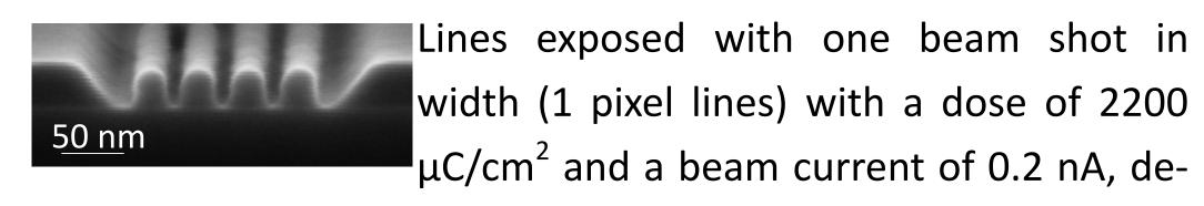
veloped in cold AR-600-546. The lines are ca. 12 nm in width. At doses below 2000  $\mu$ C/cm<sup>2</sup>, the lines were not fully developed.
