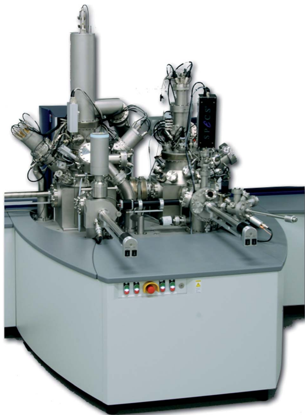
Fig. 10 ToF-SIMS 5 and Qtac 100 instruments (left and right, respectively), with their main chambers connected.
