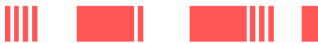
(d) Position 7: One 4 μm line in the first 50 μm trench and three in the second indicates position 7 (1+3·2).
