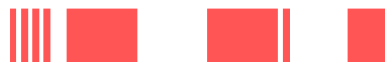
(b) Position 2: One 4 μm line in the second 50 μm trench indicates position 2.
