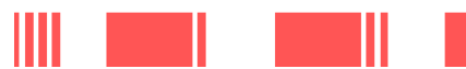
(c) Position 5: One 4 μm line in the first 50 μm trench and two in the second indicates position 5 (1+2·2).
