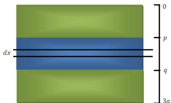
Figure 22: Intensity for electrons emerging from a layer within the surface is obtained by integrating the signal over the interval [p,q] using the exponential attenuation model e^{-x/a} .
