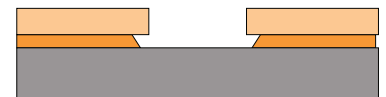
4. Develop resist and LOR. LOR develops isotropically, creating a bi-layer reentrant sidewall profile
