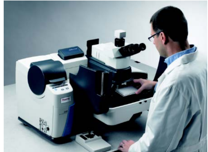
Example of a Raman microscope
