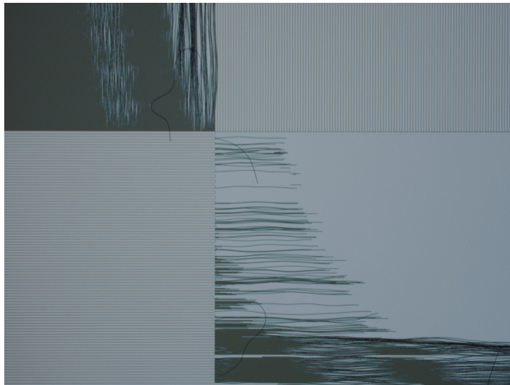
Figure 11: Macroscopic adhesion failure near centre of 24s exposure
