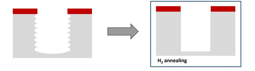
Enhanced surface mobility of Si-atoms by hydrogen annealing
