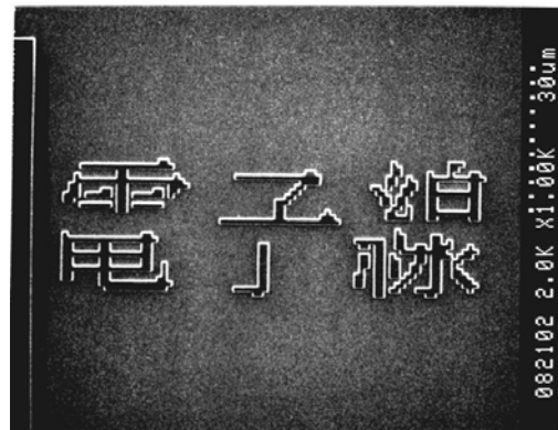
With ESPACER Charging Phenomenon on the EB Lithography Process
